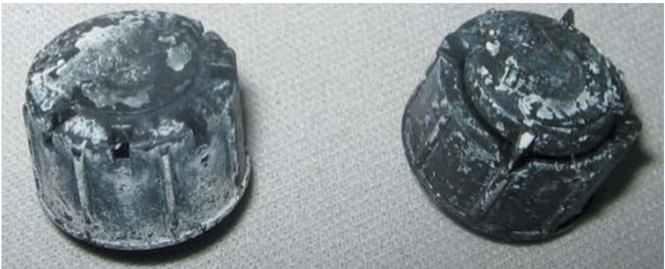
Photo 55. Salt buildup on drip emitters. Salts might be removed by flushing the irrigation lines or cleaning or replacing the emitters. (Photo by R. L. Morris.)
