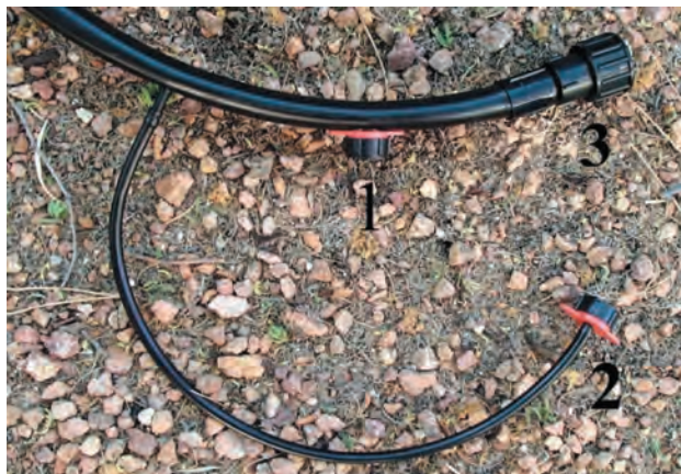
Photos 57 and 58. Drip tubing (left) showing the opening of an embedded drip emitter for the release of a precise amount of water in Lph or gph. Single emitters (right) can be connected to blank tubing, either directly (1) or by attaching them to one-quarter-inch distribution tubing (2). An end cap can be removed to flush the blank tubing which helps prevent plugging (3). (Photos by R. Morris.)
