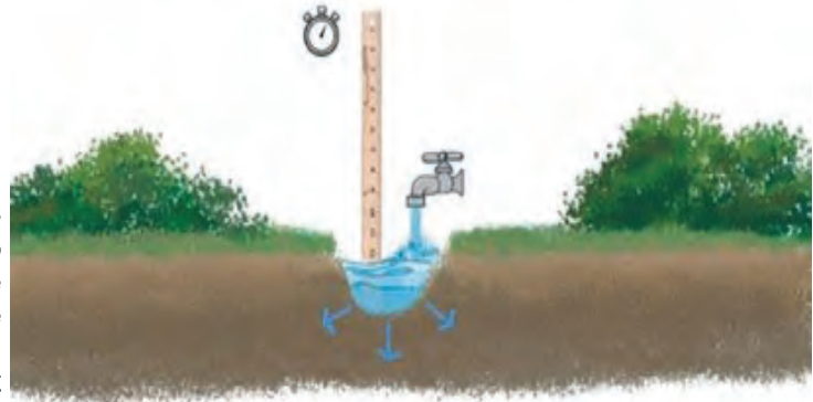
Figure 12. Percolation test to assess the rate at which water will move into a soil (drawing by N. Villeda).
