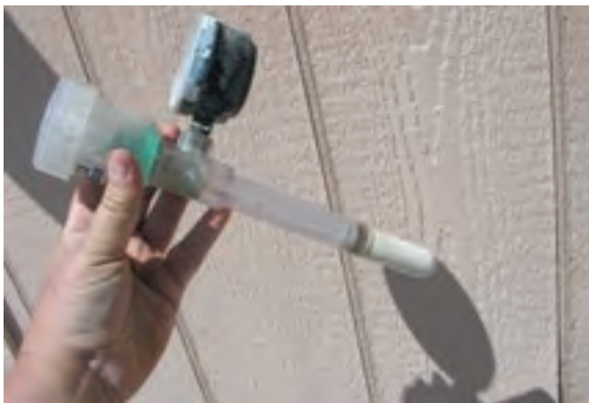
Photo 75 and Figure 20. A tensiometer is an instrument filled with water placed in direct contact with the moisture in the soil via a white ceramic tip (photo 75). Soil moisture is indirectly assessed as a vacuum (negative pressure) created on the tensiometer's internal water, which is recorded with a gauge and read in centibars of suction. It is used for assessing when to schedule irrigations. (Photo by R. L. Morris.) Placement of two tensiometers in a tree basin to help schedule irrigation events (figure 20). One tensiometer is shallow (12 inch), and the other tensiometer is placed at a depth to represent the tree's maximum rooting depth, according to its mature height (e.g., 18 inch, 24 inch, or 36 inch). (Drawing by Nancy Villeda.)
