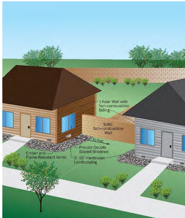
Figure 10. Examples of additional structural hardening and defensible space features where 30 feet of setback to the property line is not feasible.
